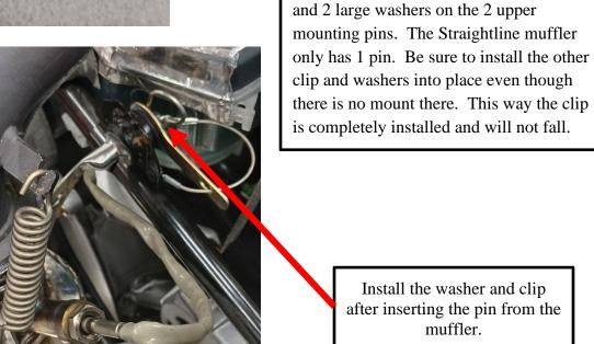
Install the washer and clip after inserting the pin from the
