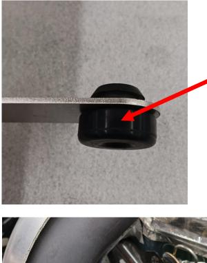
Install the stock muffler grommet as shown here. The wider part must be on the bottom. You can add a small amount of grease to ensure the grommets slide into the muffler and pins to be fully seated.
