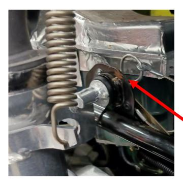
Your stock muffler used 2 hitch pin clips and 2 large washers on the 2 upper mounting pins. The Straightline muffler only has 1 pin. Be sure to install the other clip and washers into place even though there is no mount there. This way the clip is completely installed and will not fall.
