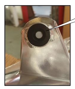
Install stock grommet into new Straightline
