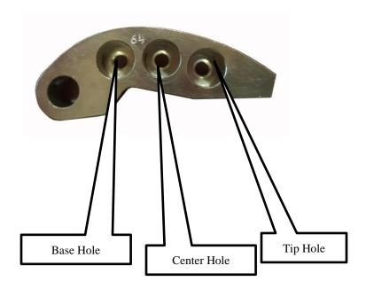
Remove the primary clutch and install the weights and primary spring. Remove secondary clutch and install new helix in proper setting, with spring. Inspect all internal clutch components for wear. If excesses wear is prevalent replace needed items.
