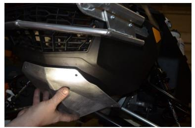
2. Drill front two dimples on stock nose cone
