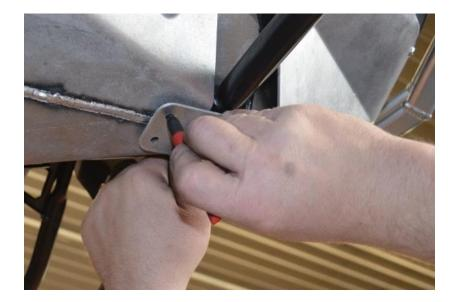
5. Using skid plate as a template drill final two holes. Then install and tighten bolts sucking skid plate up around the nose cone
