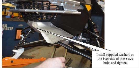
4. Using skid plate as a template push it flush with the chassis mark and drill bottom holes. Use long bolts and tighten sucking the skidplate around weld.
