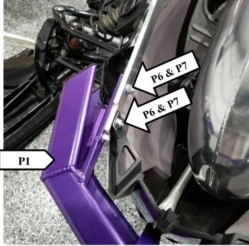
3. When installing front mount with or without skid plate, install bolt front support (P4 Qty, 1 P8 Qty 2, P7 Qty. 1) in front lower support (stock location) per pictures below.
