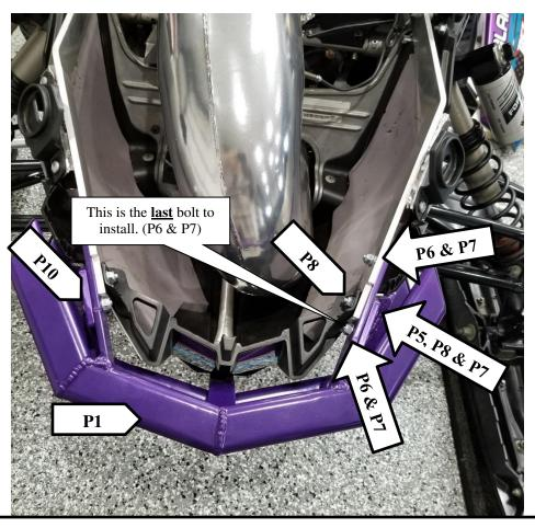
DO NOT TIGHTEN ANY BOLTS UNTIL FULLY ASSEMBLED
