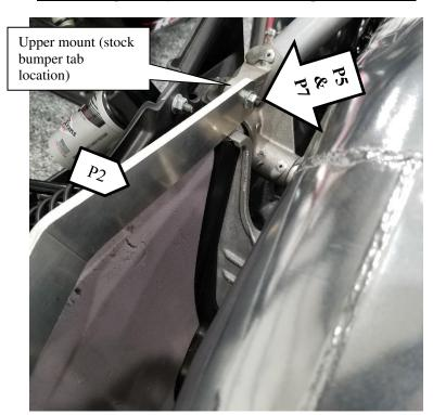
\*\*\*Do not tighten any bolts until entire bumper is assembled.
