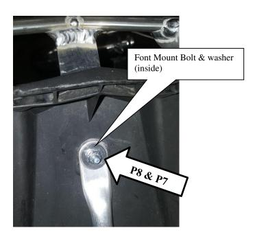
**4.** <u>Lower Wing Installation:</u> Install the lower wing (<u>P10</u>). Slide it up from the bottom and install onto the two front holes on P1. You will fasten the bottom wing using picture below for assembly. The areas that have three plates will require the longer (<u>P4</u>) bolts.
