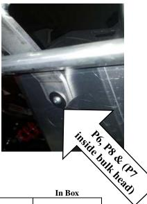
Drill Bottom holes to Straightline supplied hardware and mount lower skid plate. Removal of the exhaust may be required.
