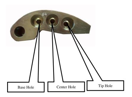
Remove the primary clutch and install the weights and primary spring. Remove secondary clutch and install new helix in proper setting, with spring. Inspect all internal clutch components for wear. If excesses wear is prevalent replace needed items.
