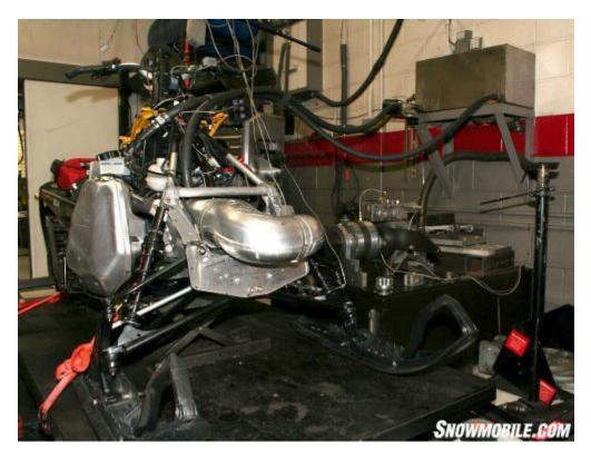
The Huff Technologies dyno is located to the right and the sled sits atop a 5000-pound lift to hoist the sled up to the dyno.
