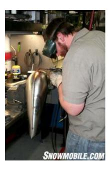
Pipe fabrication in process. At Straightline, a fabricator welds together two halves of the pipe stamping.
