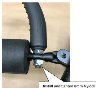
nuts on treaded stud and tighten – No need to over tighten Nylock Nut - **Repeat on opposite side**
