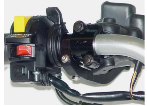
Right side view of ATV - bracket is positioned under brake lever and angles toward center.
