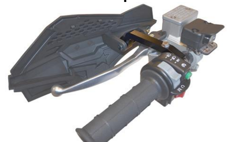
Bracket is positioned under the lever. Bracket is position
