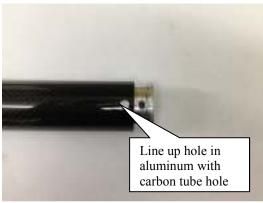
Line-up the holes before complete installation #1
