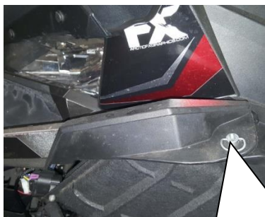
Unscrew these hood pins from both sides.
