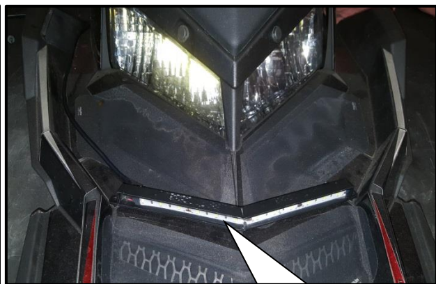
Installed LED light upper AXYS hood
