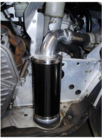
Make not of spring location on back of muffler. Be sure that the rubber grommet is in place on the base of the muffler.
