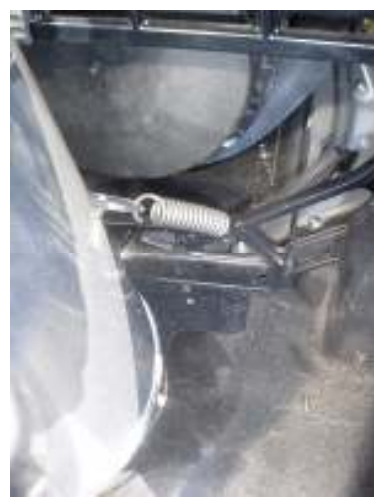
Front Lower Spring Installed #3
