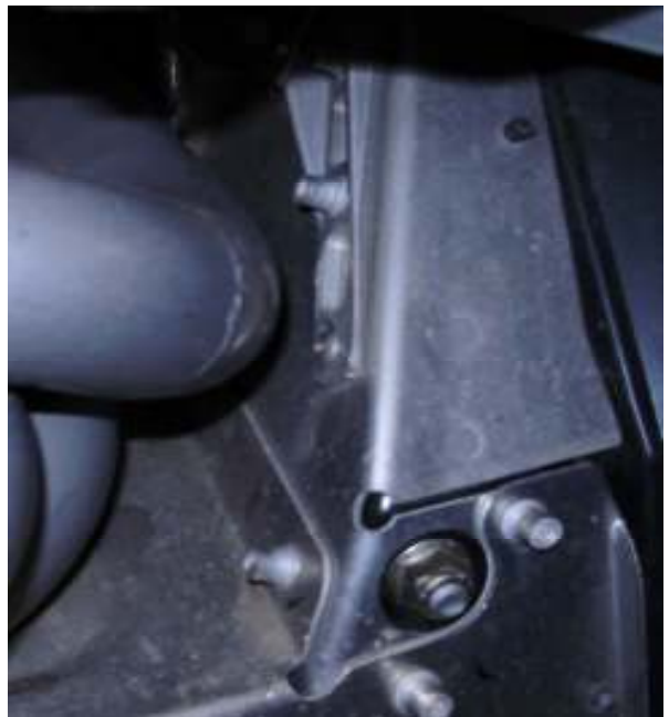
Re-install the button head screw as shown
