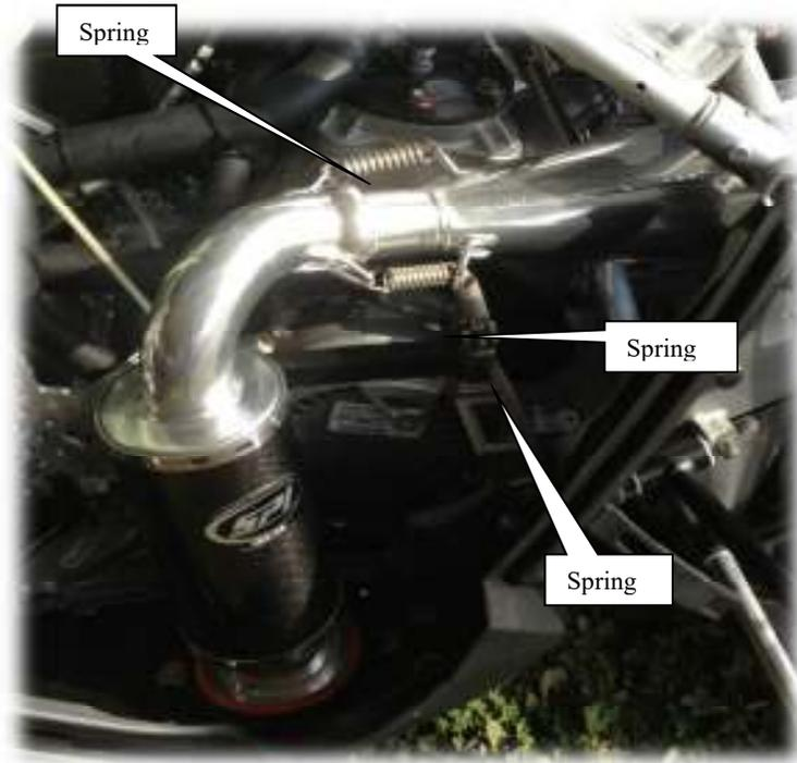
Completely installed 132-109 Polaris Carbon Fiber Muffler
