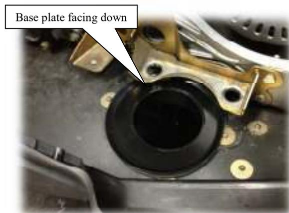
Installed base plate
