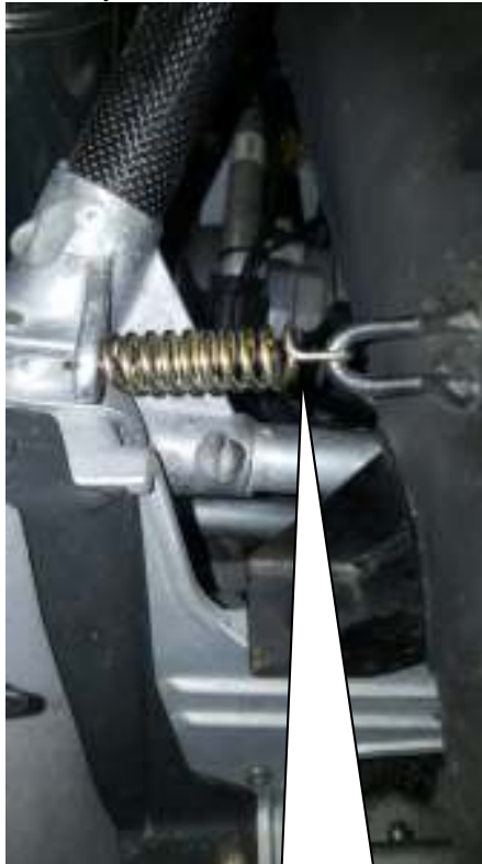
Be sure to always check spring tension to ensure proper sealing of pipe.
