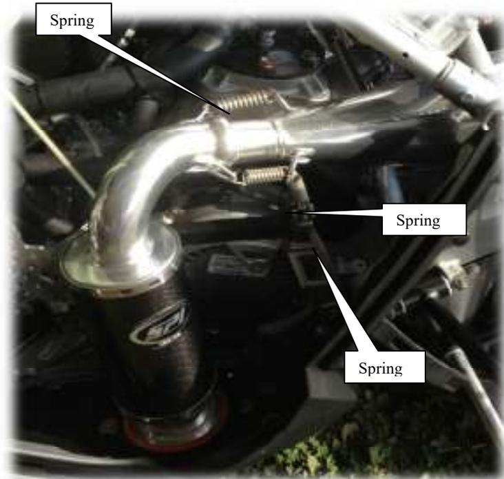
Completely installed 132-113 Polaris Carbon Fiber Muffler
