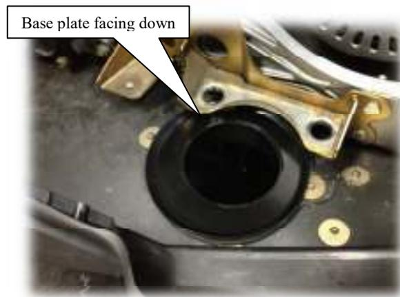
Installed base plate
