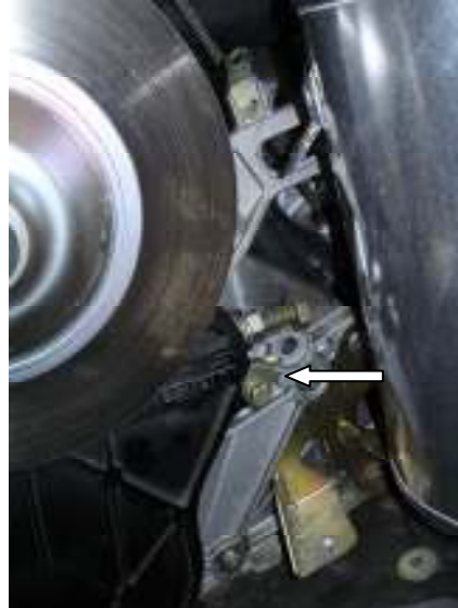
New spring clip installed under bolt
