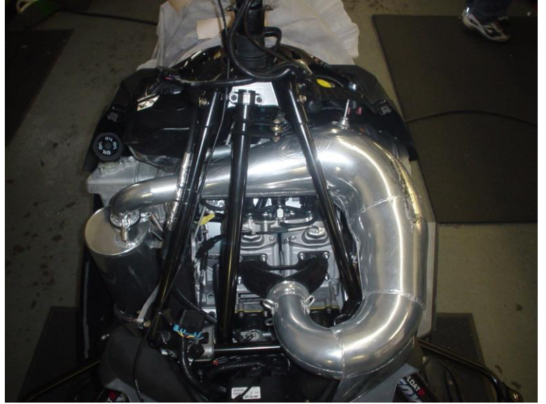
Complete Installation of the SPI Exhaust System.
