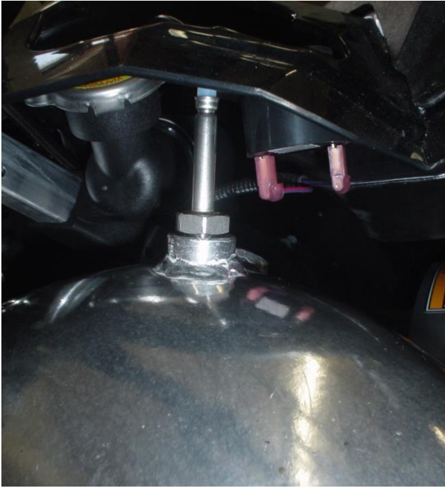
Install Heat Temp Sensor into SPI pipe as Shown.
