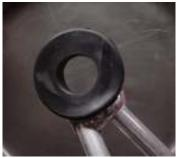
Install Straightline muffler into stock location as shown. Aligning the mounting tabs may be slightly difficult and take some time. After muffler install, re-insert the stock spacer and clip to the grommet area as shown on complete install.
