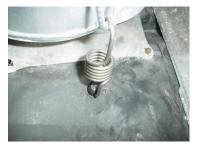
Install the 1 spring onto the other side of the silencer, and the 2 springs holding the pipe into the silencer. Silencer is ready to run.
