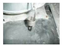
Install the 1 spring onto the other side of the muffler, and the 2 springs holding the pipe into the silencer. Silencer is ready to run.
