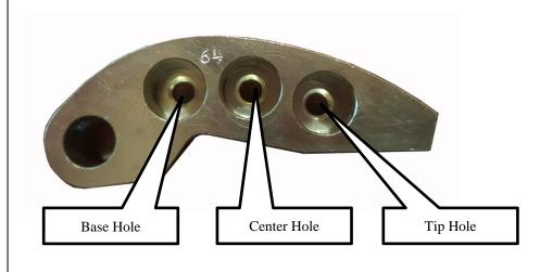
Remove the primary clutch and install the weights and primary spring. Remove secondary clutch **and install new helix in proper setting**, with spring. Inspect all internal clutch components for wear. **If excesses wear is prevalent replace needed items.**
