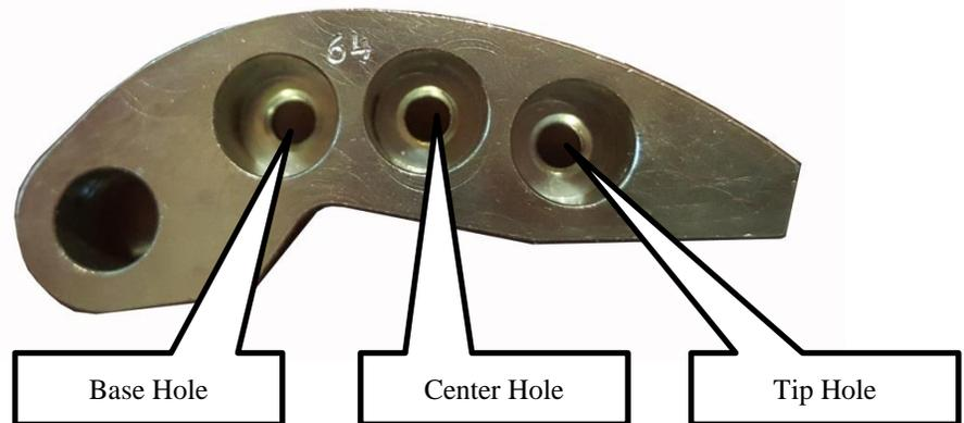
Remove the primary clutch and install the weights and primary spring. Remove secondary clutch **and install new helix in proper setting**, with spring. Inspect all internal clutch components for wear. **If excesses wear is prevalent replace needed items.**
