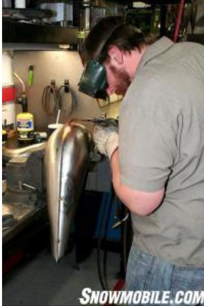
[Pipe fabrication in process. At Straightline, a fabricator welds together two halves of the pipe stamping.](#)
